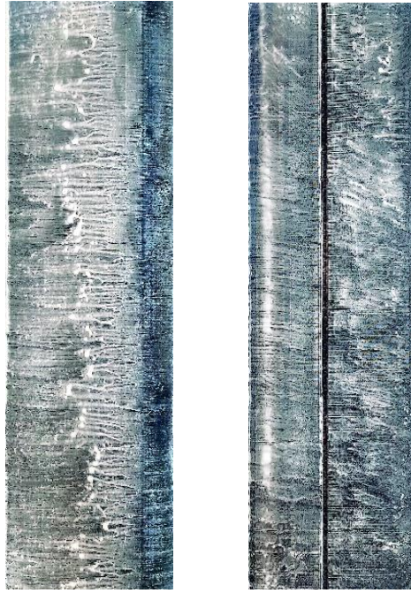
Figure 34. Top and bottom surface flow structures of the b2 airfoil models at 12 degrees angles of attack
