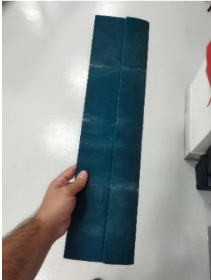
Figure 13. Airfoil with gluing and sanding operations realized
