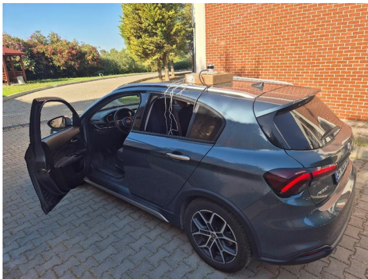
Figure 2. Ouster-OS1 LIDAR mounted on top of the vehicle to collect data
